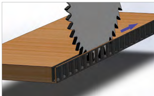
Vertical sawing of mortice
