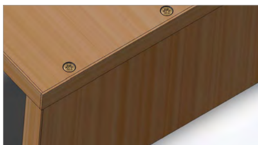
Screwed corner of carcass
