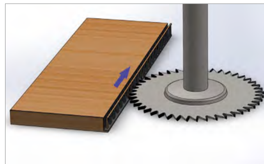
Horizontal sawing of mortice
