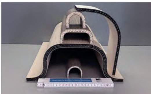
Formed elements with a minimum inside radius of r = 15\text{ mm}
