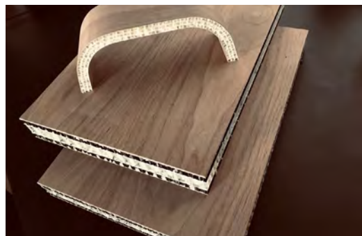
Sandwich molded panels from RENOLIT GORCELL.
