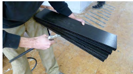
Edge cleaning with compressed air
