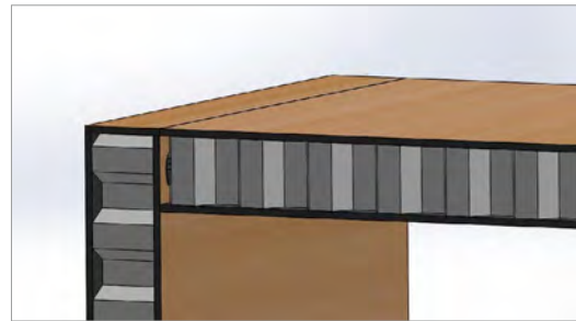
RENOLIT GORCELL carcass corner bonded abutted
