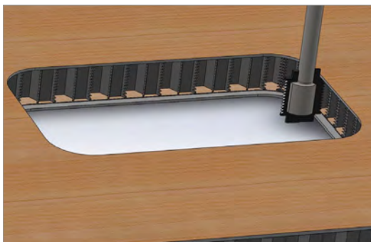
Milling a groove into the core
