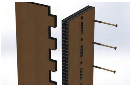
RENOLIT GORCELL panel milled T-joint
