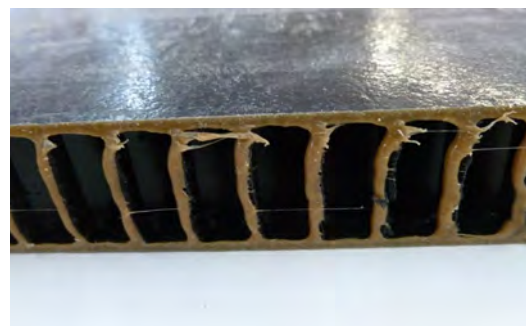
Application of adhesive in counter direction
