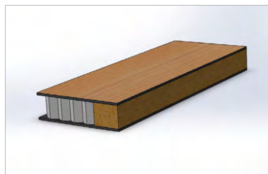
Edge trim with rigid foam material
