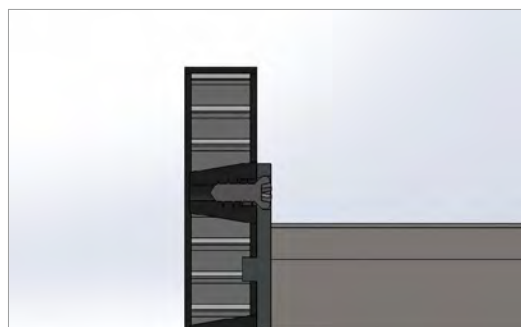
Wardrobe rail support without catch pins
