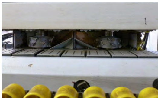
Joint cutters on an edge gluing machine
